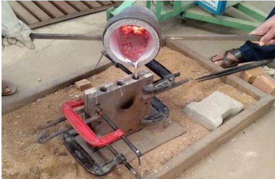
Figure 2.3: Pouring of metal matrix composite.
